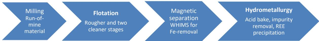
Figure 2: Simplified Lofdal process flowsheet for direct flotation of run-of-mine material
